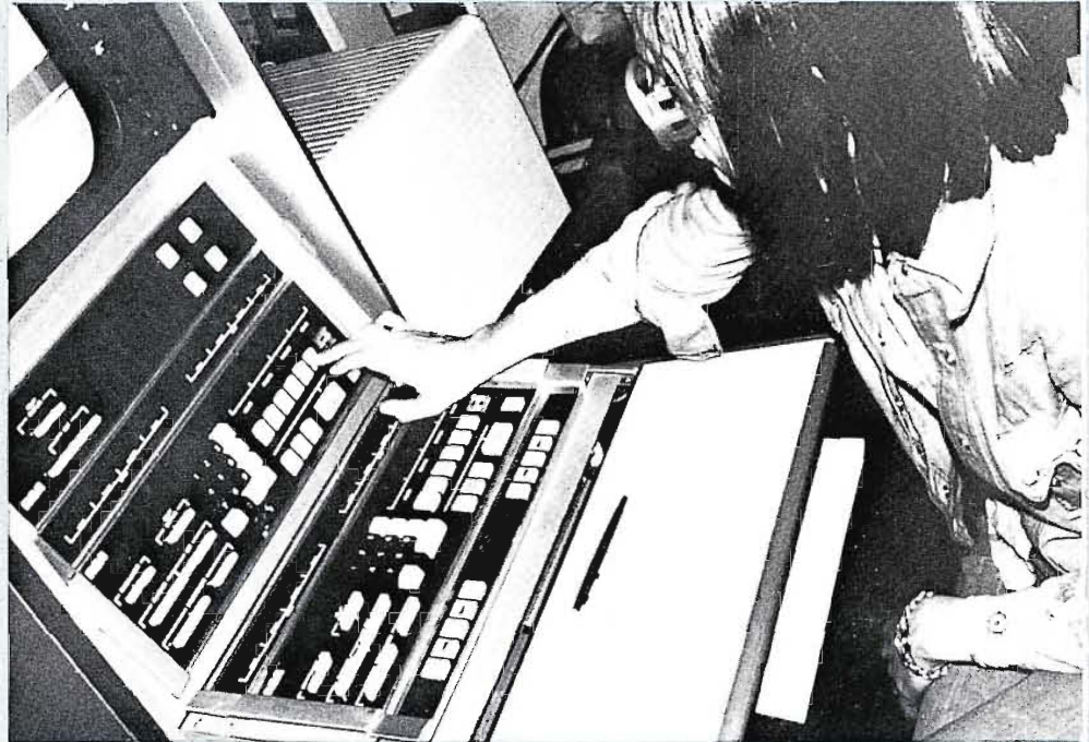
With the aid of RCA's Time Code Editor, VTR Supervisor Jacqueline Jeannert uncomplicates the video tape editing procedure. Identifying each frame of information in hours, minutes, seconds and frames, the TCE lends speed, accuracy and flexibility to the whole process.
