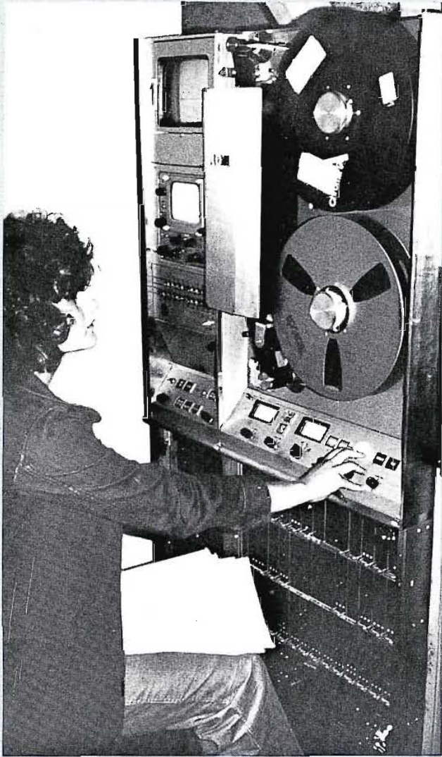
A VTR operator monitors a TR-60 producing the high-quality master tapes necessary for final assembly work.
