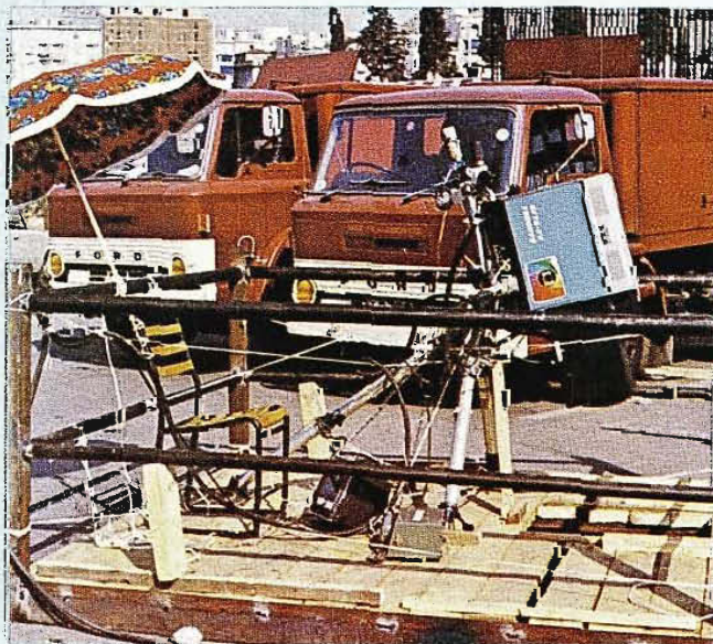
This platform for mounting TK-44 camera looks innocuous enough on terra firma. During the Diving Championships, it was suspended from a crane, 180 feet above ground, shooting down on the 100-foot diving platform. The parasol provided a small creature comfort for the cameraman on his precarious perch. Red trucks in background are power generators.
